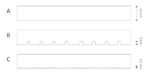
5- 10 YEARS MONITORING - BASED ON HALF-A-YEAR MONMITORING OF WOOD MOISTURE WE CAN CONCLUDE, THAT THE GROOVES GREATLY SHORTEN THE TIME WHEN THE HUMIDITY OF THE TILES IS SUITABLE FOR DECAY. THE SLOTS WORK EVEN BETTER IF SHINGLES ARE PROTECTED WITH WATER SUSPENSION OF WAX.
